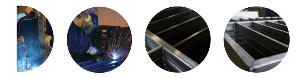
At Continental Wire Cloth Robotics are used to produce frames with the latest robotic welding technology. In addition, we use laser cutting and punch presses to ensure continuity in production resulting in high quality screens.
